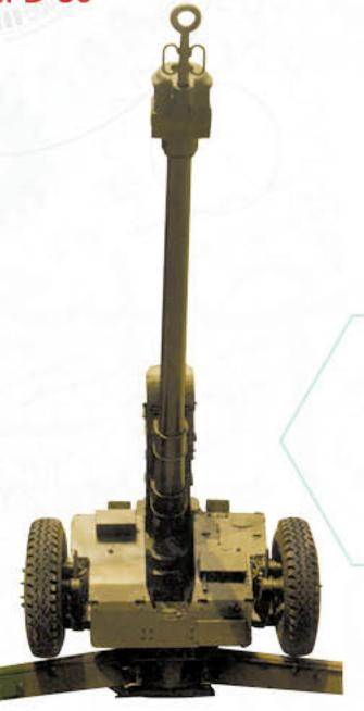
It's towed for direct firing at movable and stationary targets by optical sight, its panoramic telescope and the range quadrant. It's not only used for firing from masked position, but also for direct firing.
